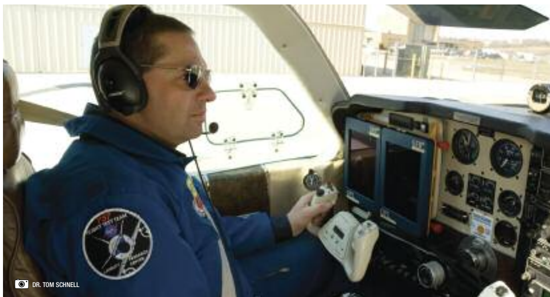
Airborne simulation testing of synthetic vision system for enhancing operator visuals and situational awareness. Study conducted by the Operator Performance Laboratory (OPL) at the University of Iowa.
